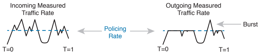
Figure 18-18 Effect of a Policer and Shaper on an Offered Traffic Load
